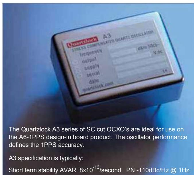
The Quartzlock A3 series of SC cut OCXO's are ideal for use on the A6-1PPS design-in board product. The oscillator performance defines the 1PPS accuracy.
