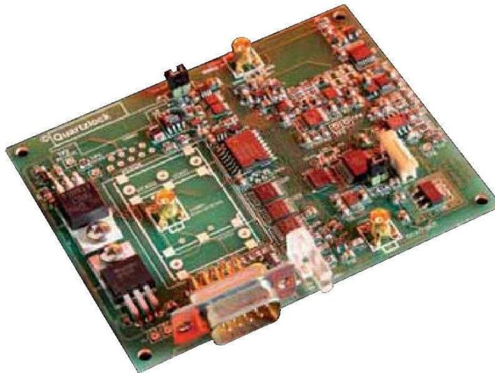
The A6-CPS digital phase locked loop (PLL) provides a low noise, very high short term stability filtered output which can be customised to a specific application.
