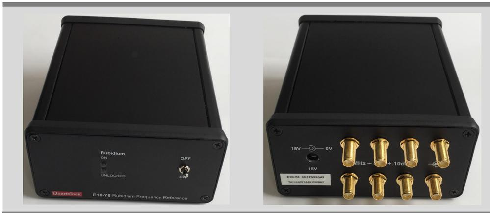
Compact simple to install low noise multi-output atomic frequency reference for use as a general purpose 10MHz rubidium frequency standard. This very low noise rubidium frequency reference will enable up to eight separate instruments to be referenced. This frequency standard benefits from having Quartzlock's SMAC (Sub Miniature Atomic Clock), and very low noise distribution amplifier technology built in.
